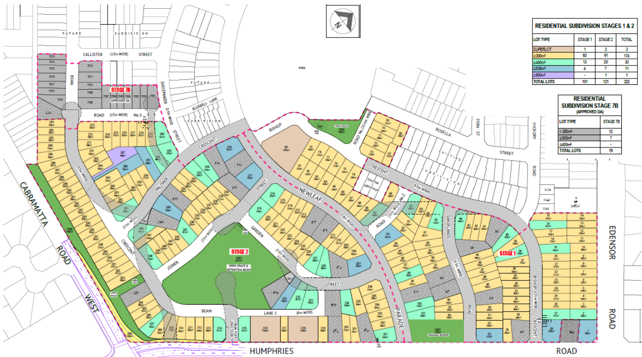
Figure 2 – Proposed Subdivision Plan extract showing the proposed layout of new roadways, allotments and open space areas.
